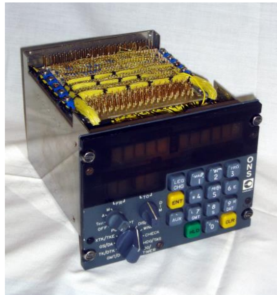
Figure 14.8 Typical control display unit
